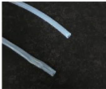
[Checking for damage to the tube]
